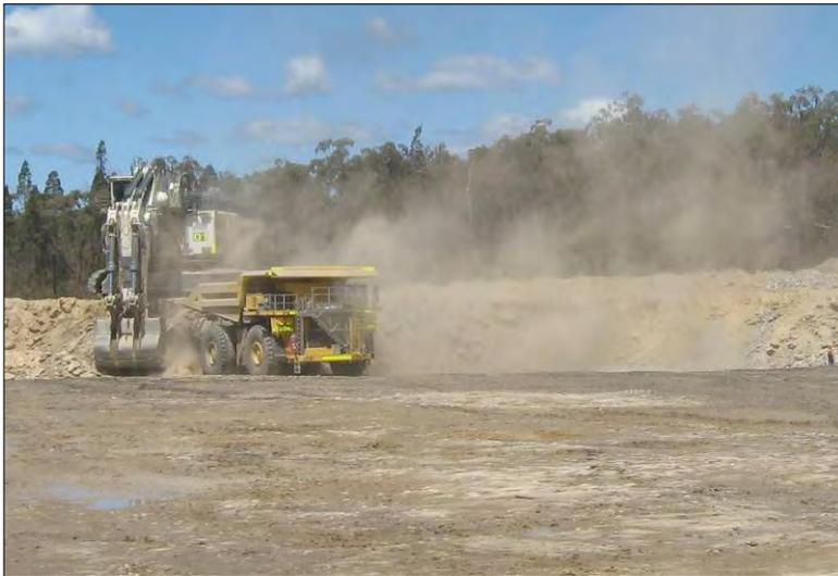
Photo 13: Excavation of dry soil layer and overburden (Dec 09)
