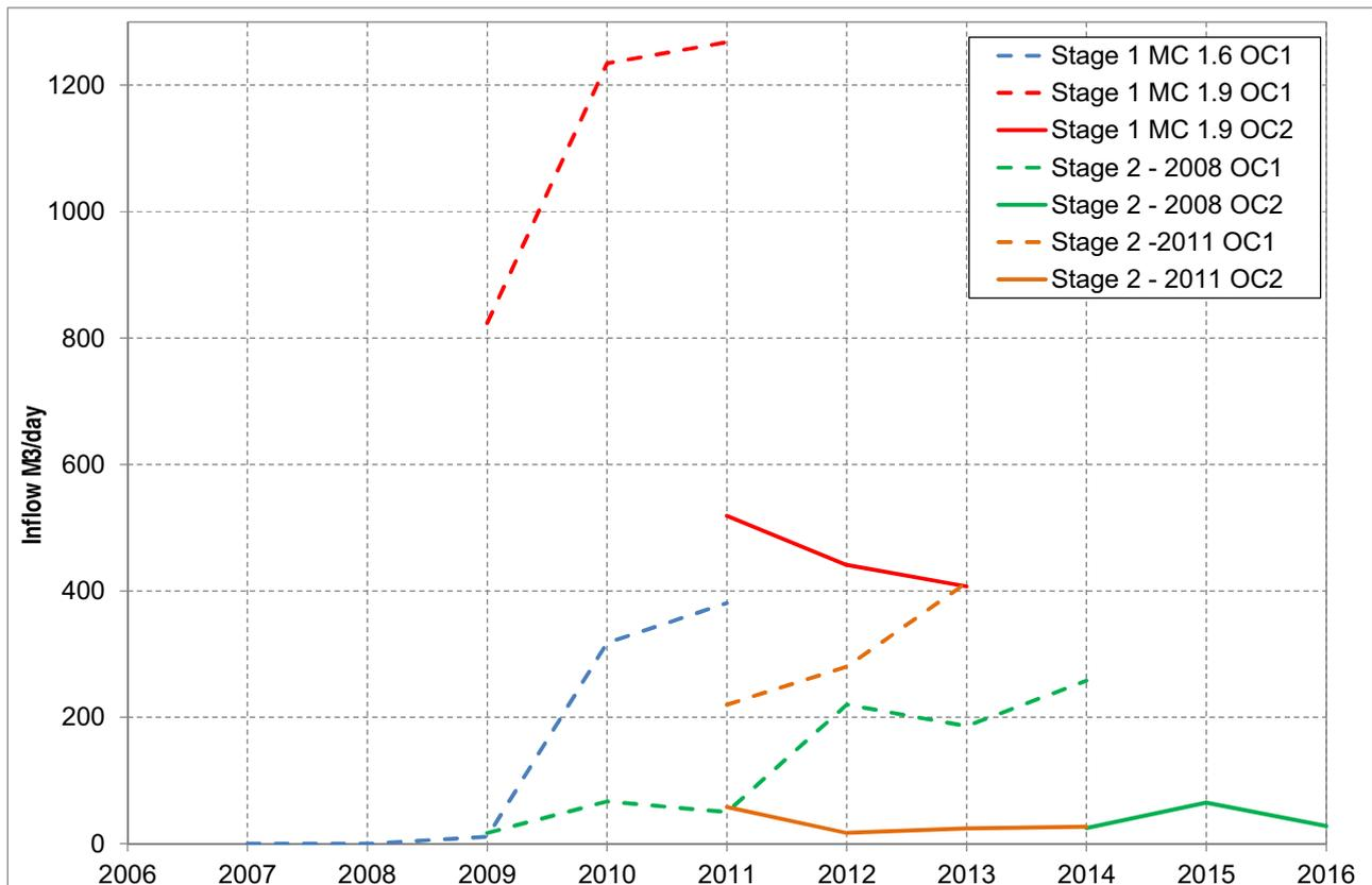
**Figure 26: Mine inflow rates for Open Cut 1 and 2 from different Stage 1 and 2 Models**
