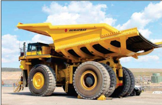
Plate 1 Haul truck fitted with Duratray
