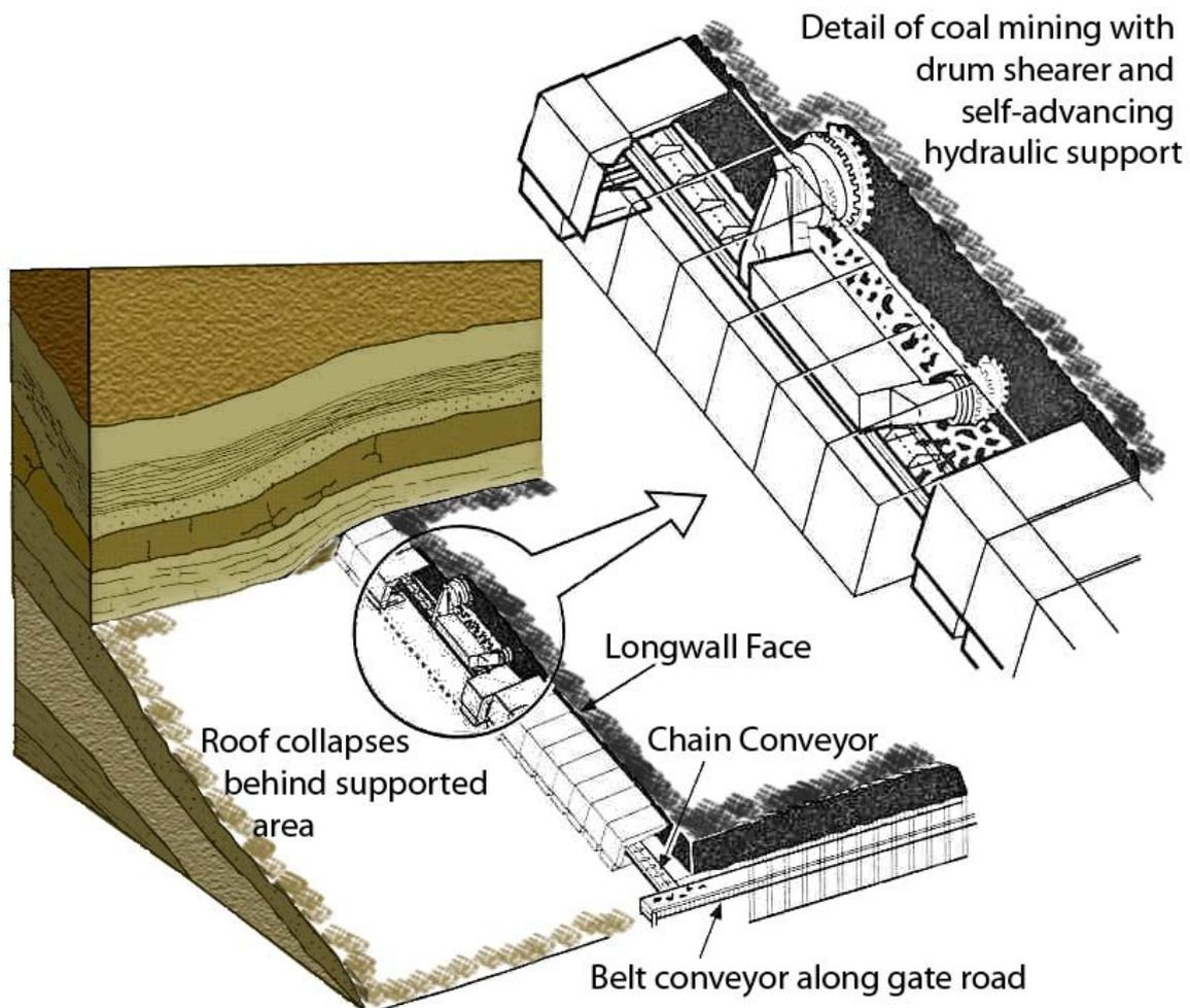
**Figure 4.13: Schematic diagram of a longwall mining operation.**
