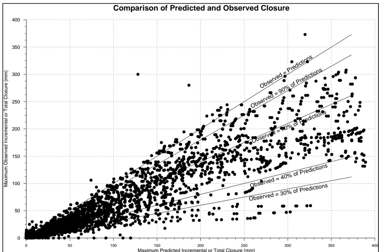
Fig. 3.4 Plot of Predicted versus Observed Closure
