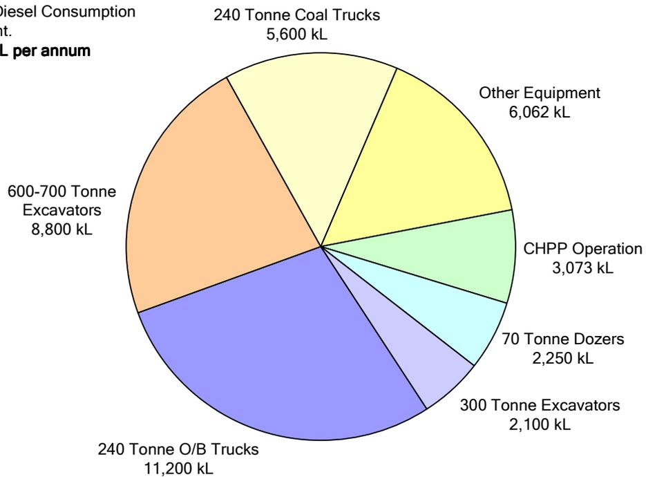
**Figure A3: Projected Diesel Consumption for major equipment**
