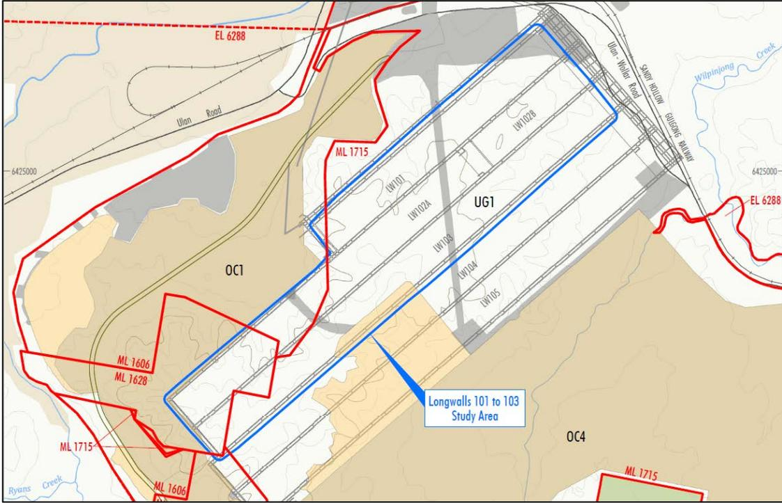
FIGURE 1. UG1 Longwalls 101 to 103 Extraction Plan Current Layout
