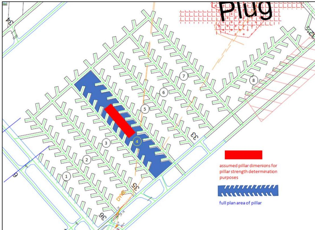
**FIGURE 4. Illustration of Full Remnant Pillar Plan Shape and Dimensions As Compared to Assumed Pillar Dimensions for Strength Determination Purposes**
