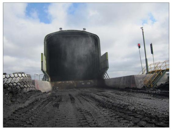
PLATE 5 Water sprays in operation on ROM dump hopper
