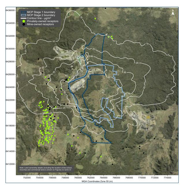
Figure 5-1: Predicted maximum 24-hour average PM<sub>10</sub> concentrations due to emissions from the Modification
