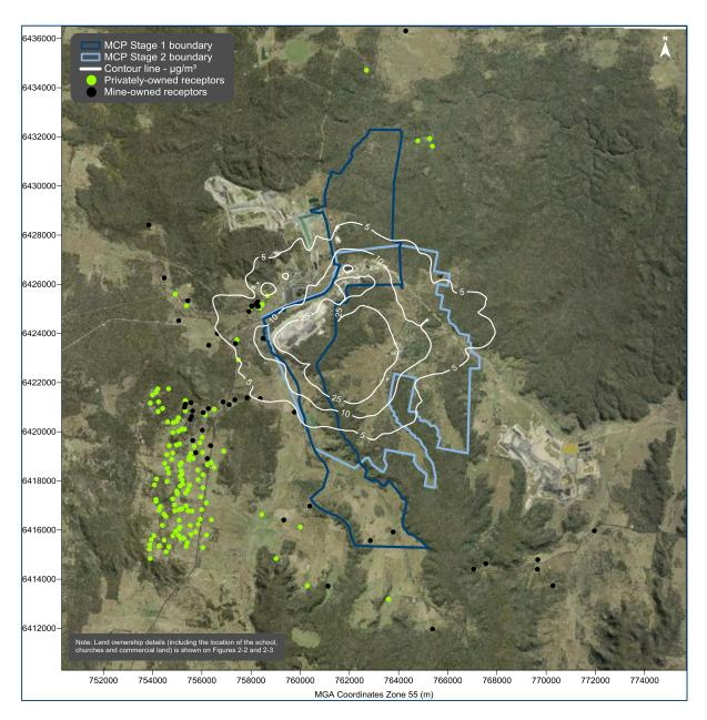
Figure C-1: Predicted maximum 24-hour average PM<sub>2.5</sub> concentrations due to emissions from the Modification
