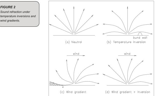
Figure 2 shows that sound rays can be refracted over a barrier (usually a bund wall or small hill) during a temperature inversion, increasing noise levels in the 'shadow zone'.
