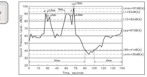
The signal in Figure 3 has a duration of 2.5 minutes (ie 150 seconds) with noises occurring as follows:
