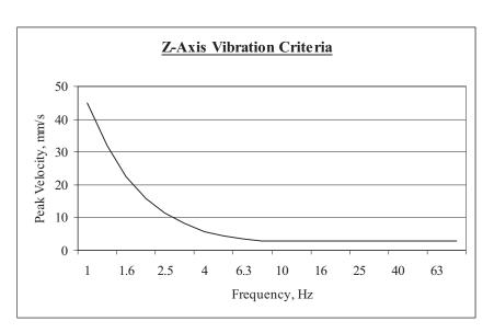
As train-induced ground vibrations typically comprise frequencies greater than 10Hz, and the vertical vibration criteria are more stringent than the horizontal vibration criteria, a maximum allowable vertical vibration velocity of 2.82mm/s applies.
