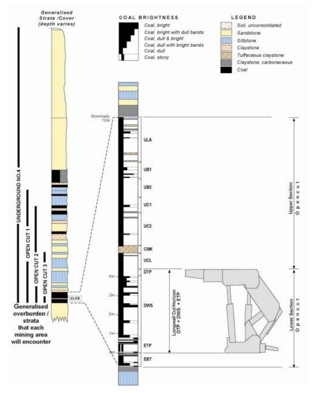
Figure 4.2: Proposed working sections of Ulan Coal for Underground and Open Cut operations.
