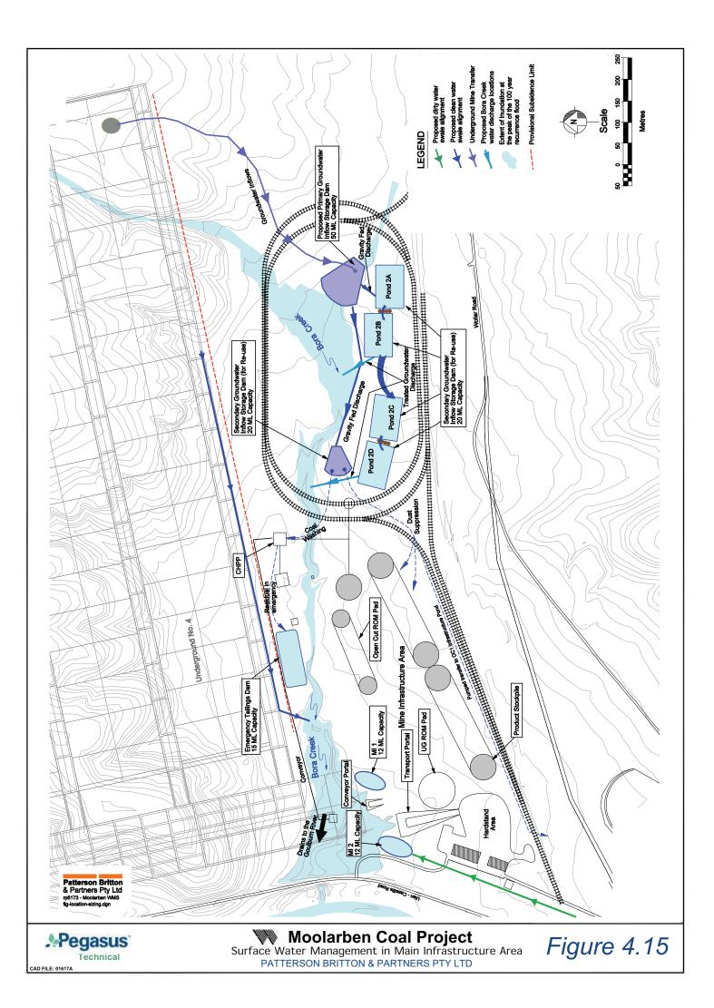
• Progressive downstream discharge of treated groundwater make through each of Groundwater Treatment Ponds 2A, 2B, 2C and 2D. Testing of treated groundwater in Pond 2C and subsequent discharge to Bora Creek/Goulburn River once acceptable water quality is achieved.
