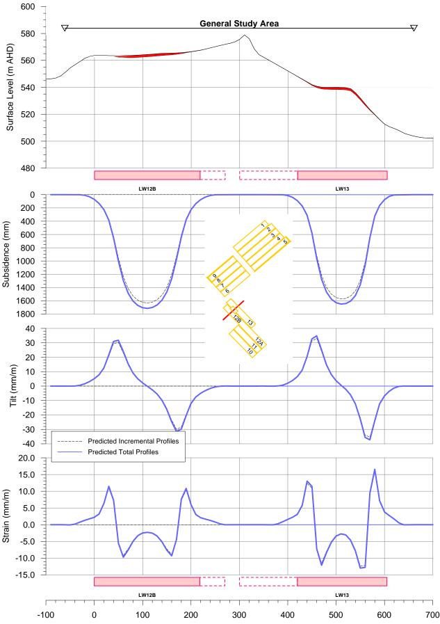
I:\Projects\Woolarben\WSEC353 - Stage 2 MCP\Subsdata\Impacts\Drainage Lines\Fig C.05 Moolarben Drainage Lines - DL1 - Initial and Subsided surface levels Landscape.grf.....27-Jul-11 Moolarben Coal Project - Stage 2, Underground 1 and Underground 2 - Longwalls 1 to 13 Profiles of Initial and Subsided Surface Level, and Predicted Subsidence
