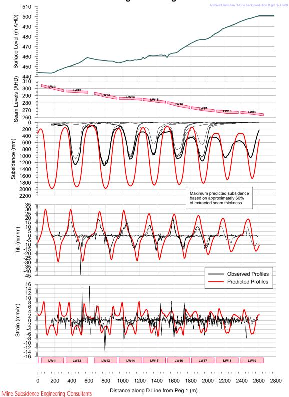
Fig. 3.6 Ulan Mine Longwalls 11 to 19 Monitoring Results along Monitoring Line D in the Ulan Seam
