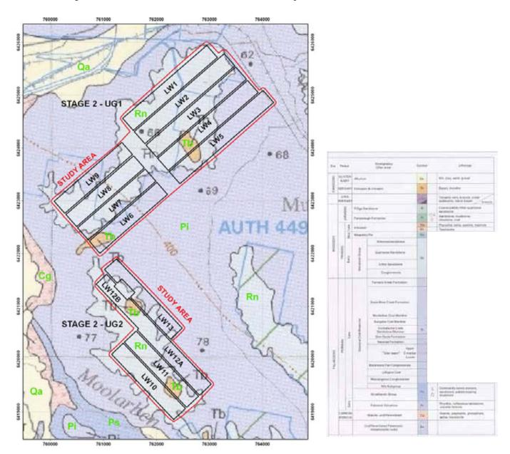
Fig. 1.3 Surface Geological Map Showing Proposed Longwalls 1 to 13 and the Study Area (Source-1:100000 Western Coalfield Map)
