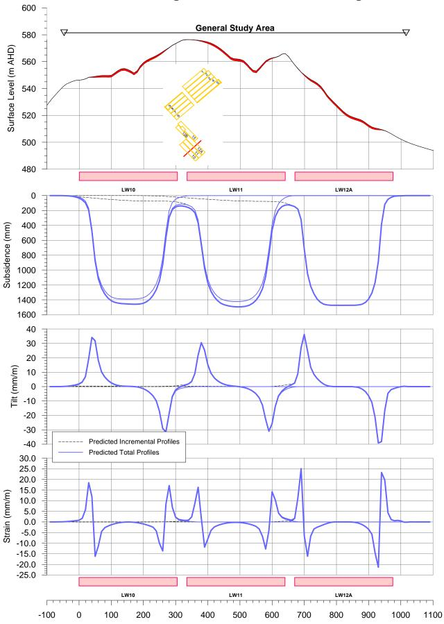
Distance along Prediction Line from the Tailgate of Longwall 10 (m) Fig. C.03
