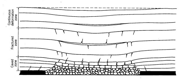
Fig. 5.3 Zones in the Overburden According to Peng and Chiang (1984)
