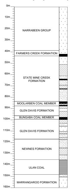
Fig. 1.4 Stratigraphic Column (based on WMLB117)
