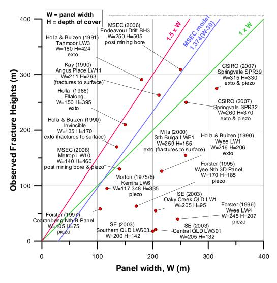
Fig. 5.5 Observed Fracture Heights versus Panel Width
