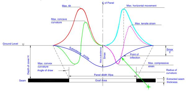
Fig. 3.2 Typical Profiles of Systematic Subsidence Parameters for a Single Longwall
