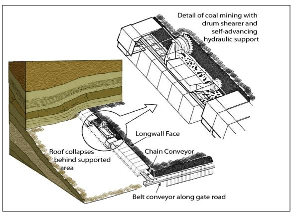
Figure 4.3 Schematic diagram of a longwall mining operation
