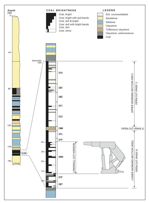
Figure 4.2 Indicative working sections for the Ulan Seam for underground and open cut operations
