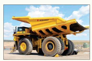
Plate 1 Haul truck fitted with Duratray
