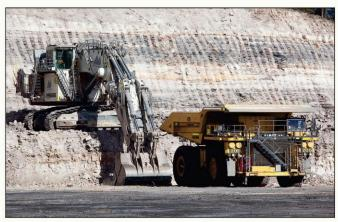
Plate 2 Excavator shielded by pit wall
