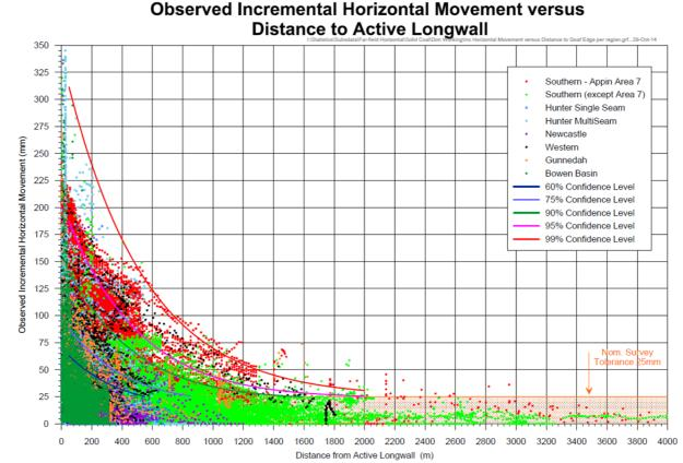
Fig. 3.13 Observed Incremental Far-Field Horizontal Movements (mm) from many regions in NSW plotted against the distance to the nearest edge of the mined panel (m)
