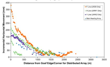
Fig. 3.16 Observed Incremental Far-Field Horizontal Movements at UCM (Mills)
