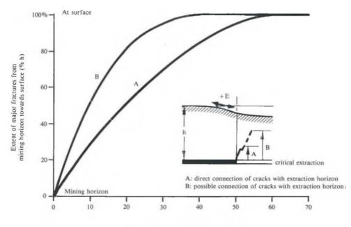
Predicted maximum tensile strain (+E), mm/m
