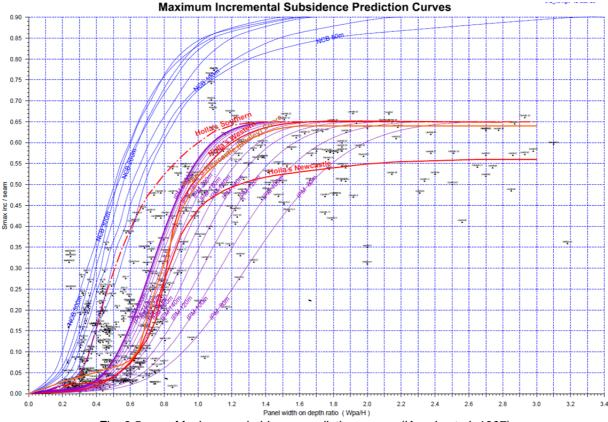
Fig. 3.5 Maximum subsidence prediction curves (Karmis et al, 1987)
