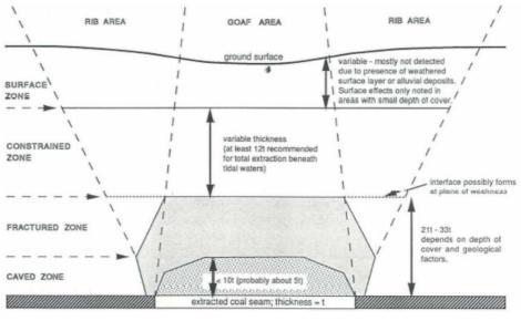
Fig. 4.7 Zones in the Overburden according to Forster and Enever (1992)
