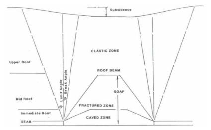
Fig. 4.8 Zones in the Overburden according to McNally et al (1996)
