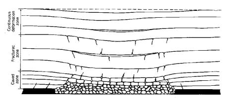
Fig. 4.4 Zones in the Overburden According to Peng and Chiang (1984)
