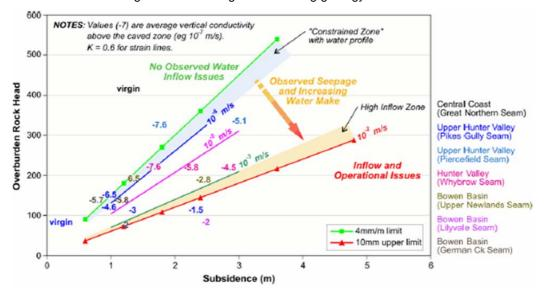
Fig. 4.11 Average Overburden Conductivity characteristics relative to subsidence and depth criteria (Gale, 2007)
