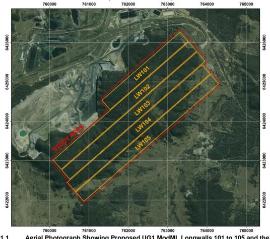
Fig. 1.1 Aerial Photograph Showing Proposed UG1 ModML Longwalls 101 to 105 and the UG1 Study Area
