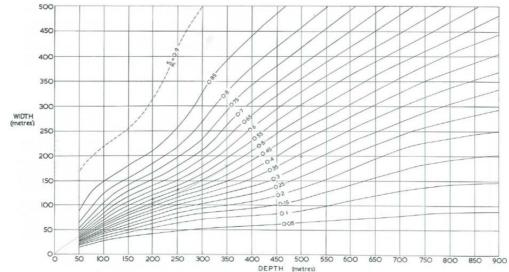
Fig. 3.4 Maximum subsidence factor prediction curves based on Width and Depth (SEH, 1966 & 1975)
