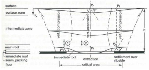
Fig. 4.3 Zones in the Overburden according to Kratzsch (1983)
