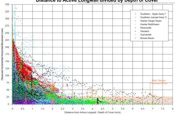
Observed Incremental Horizontal Movement versus Distance to Active Longwall divided by Depth of Cover
