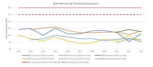
**Figure 5 Blast Monitoring Trending Overpressure**
