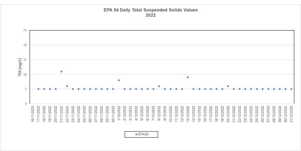
Figure 22: EPL LDP 54 Total Suspended Solids (mg/L)
