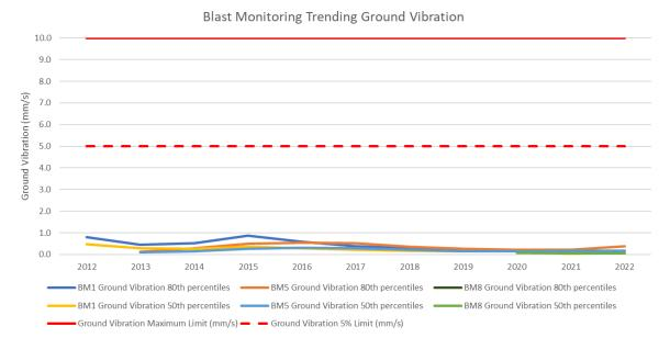
**Figure 4 Blast Monitoring Trending Ground Vibration**
