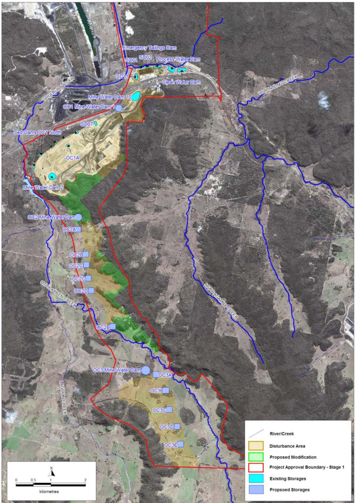
**Figure 7: Stage 1 Surface Water Management Infrastructure within Open Cuts**
