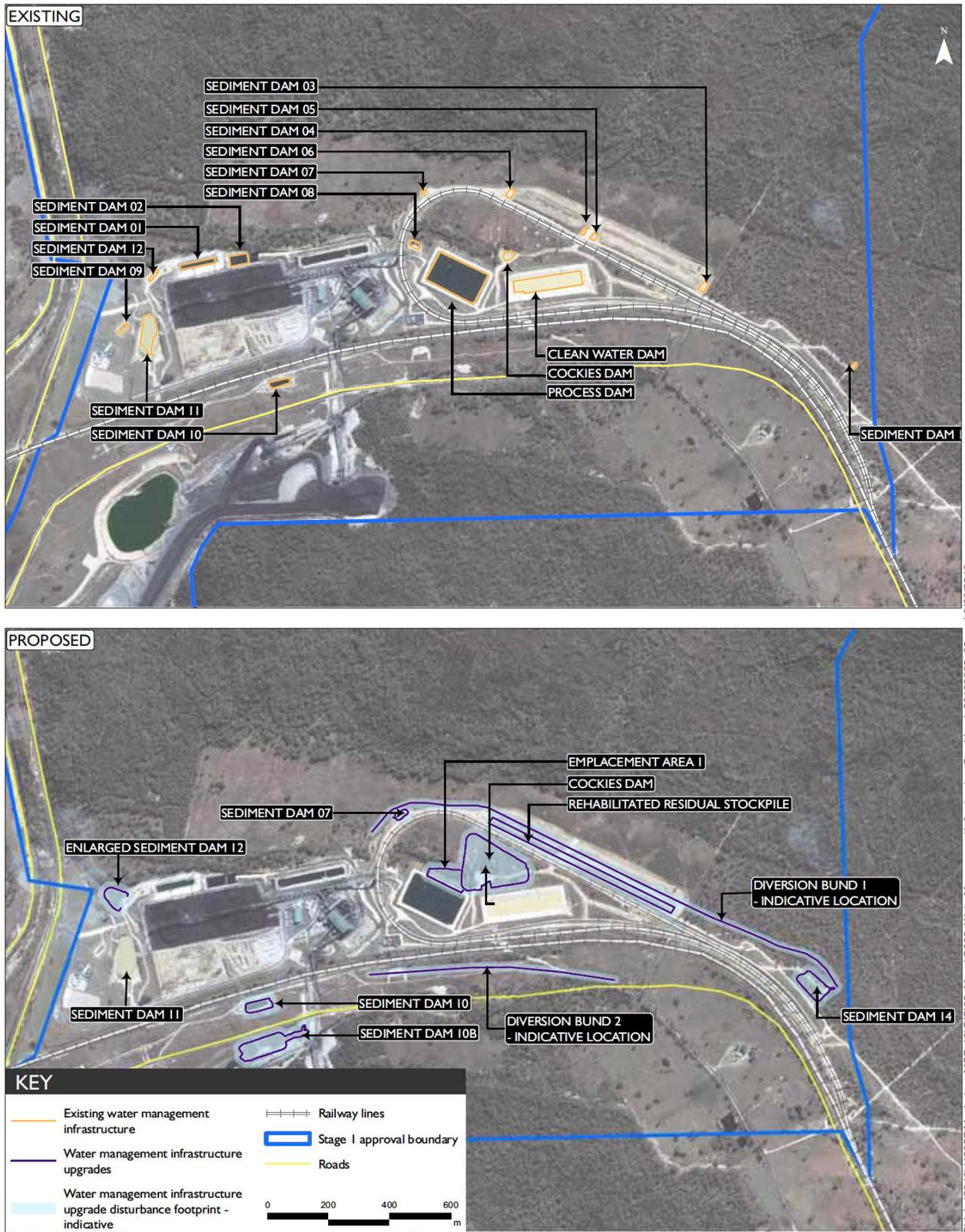
**Figure 6: Existing and Proposed Stage 1 Surface Water Management Infrastructure**
