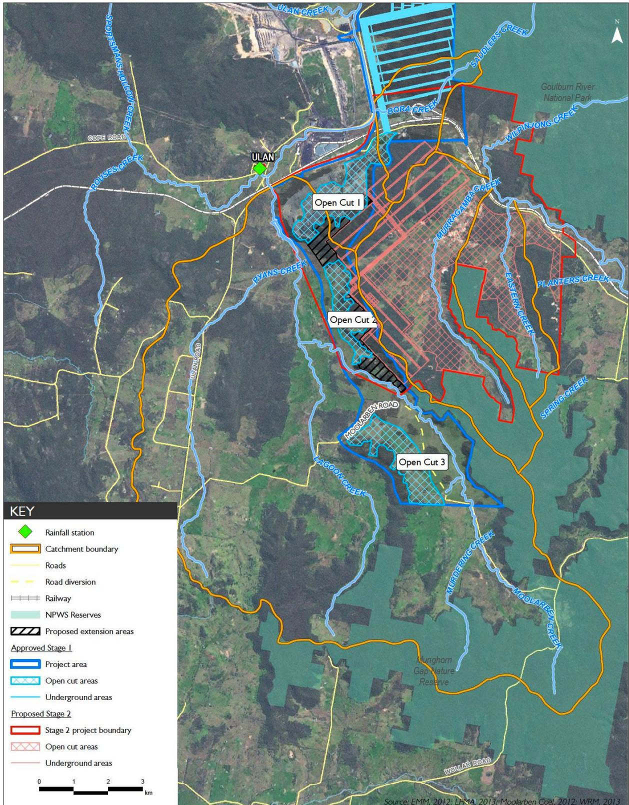
**Figure 13: Local Drainage Network**
