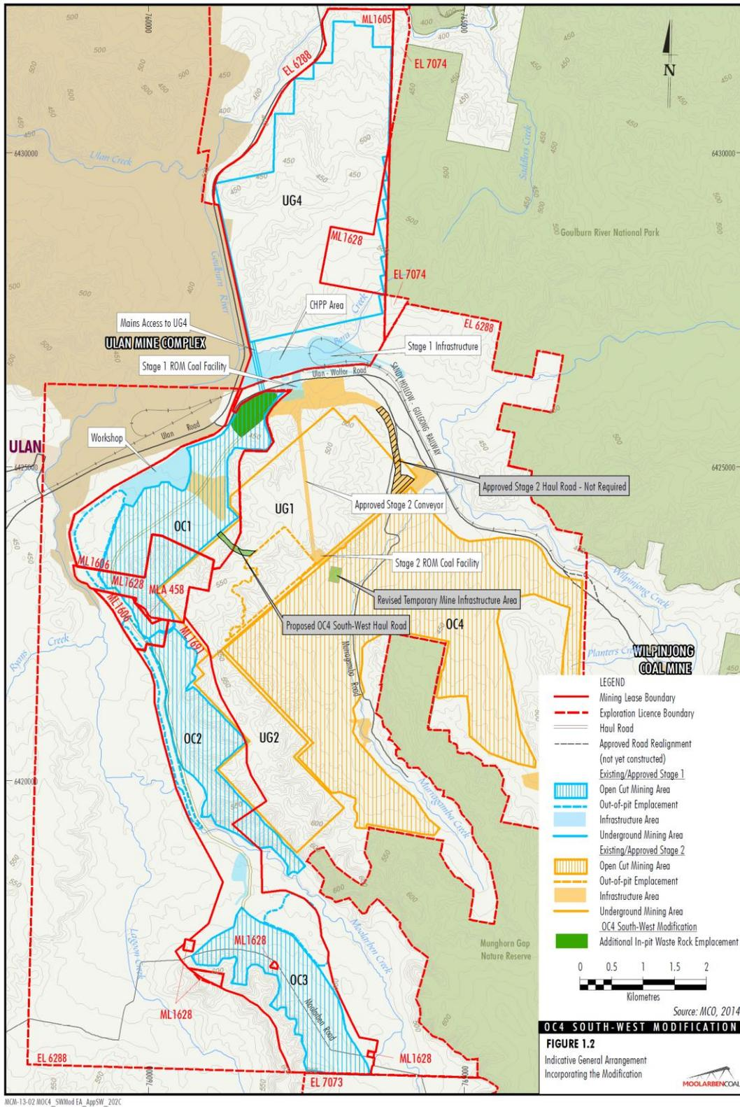
Figure 1.2 - Indicative General Arrangement Incorporating the Modification
