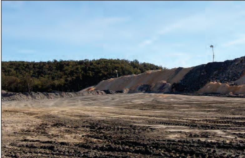
Plate 3 Overburden dump area shielded by side of waste emplacement
