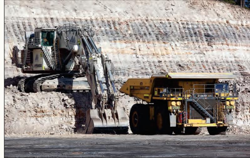
Plate 2 Excavator shielded by pit wall
