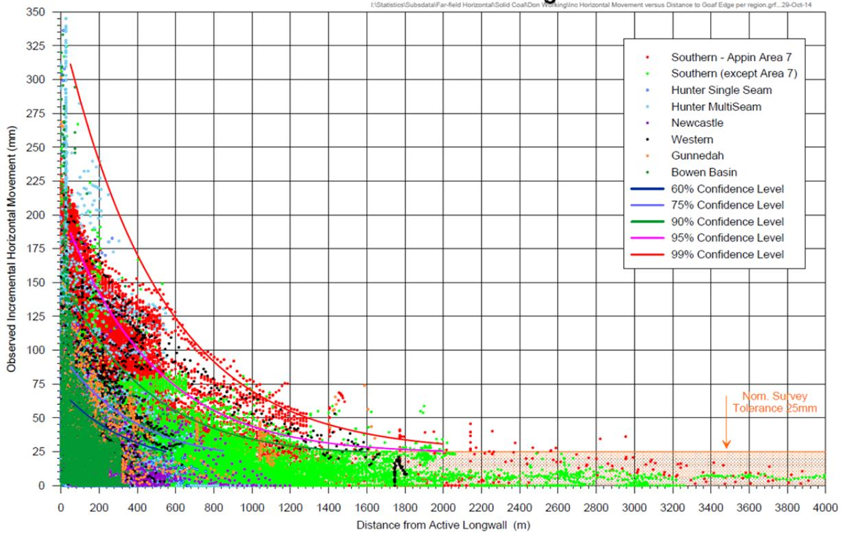
**Fig. 3.13** Observed Incremental Far-Field Horizontal Movements (mm) from many regions in NSW plotted against the distance to the nearest edge of the mined panel (m)
