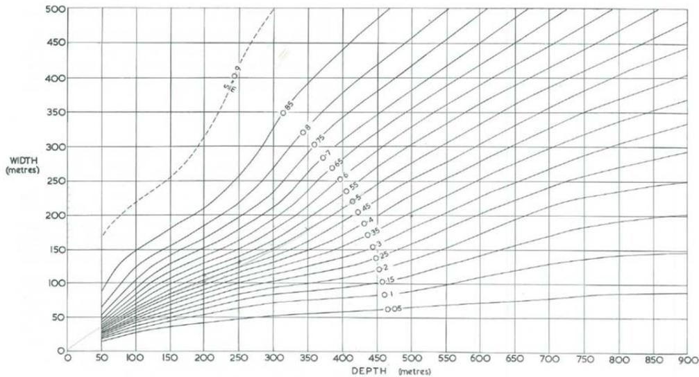
Fig. 3.4 Maximum subsidence factor prediction curves based on Width and Depth (SEH, 1966 & 1975)
