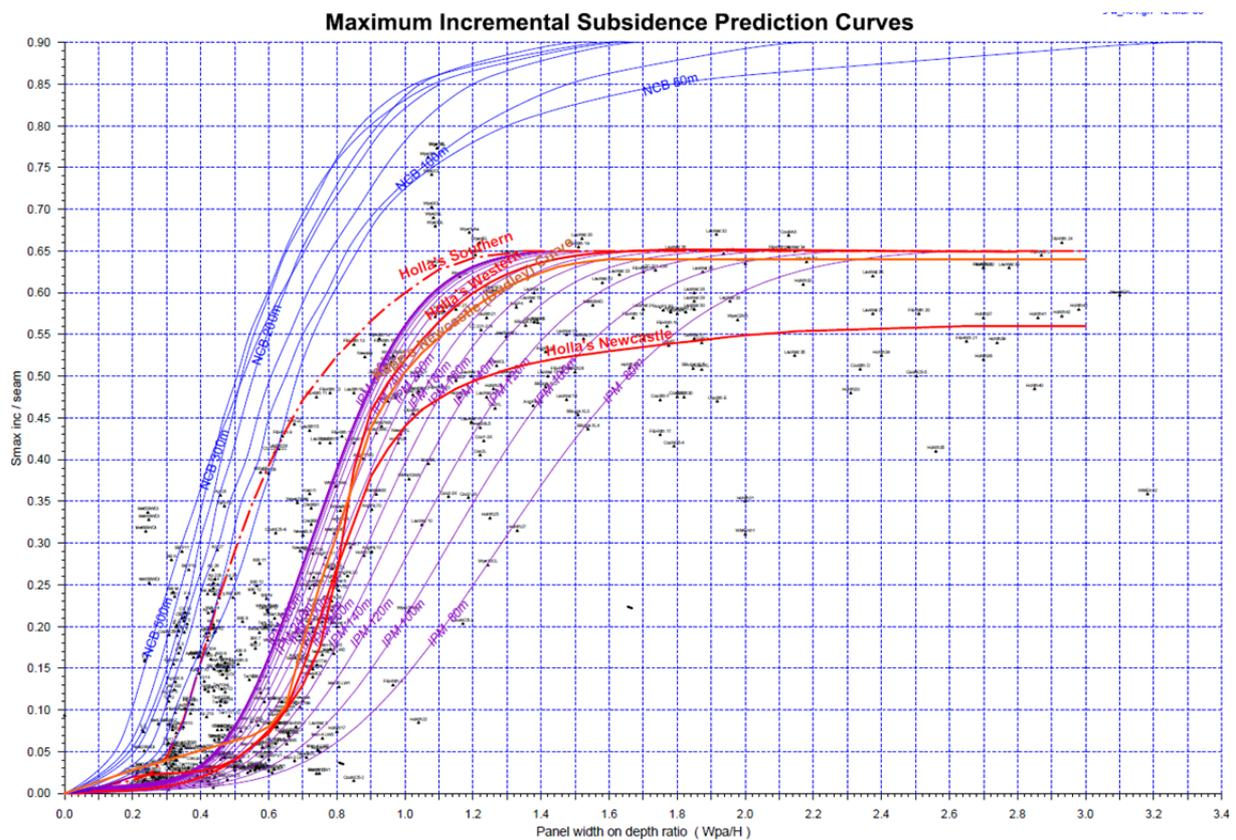
Fig. 3.5 Maximum subsidence prediction curves (Karmis et al, 1987)
