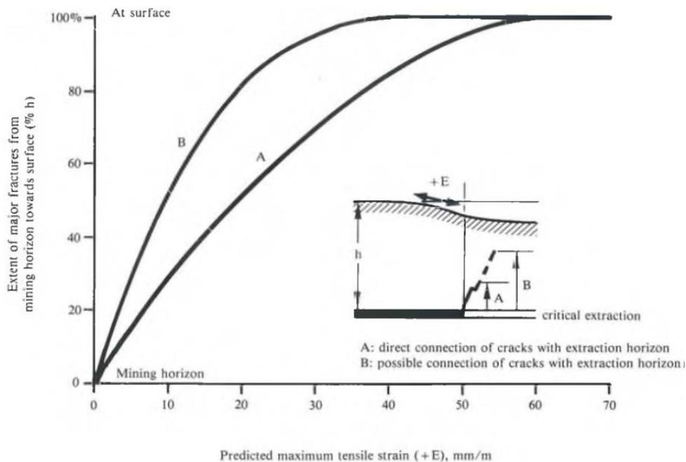
**Fig. 4.6 Extent of Major Fractures from the Mining Horizon (Whittaker and Reddish, 1989)**
