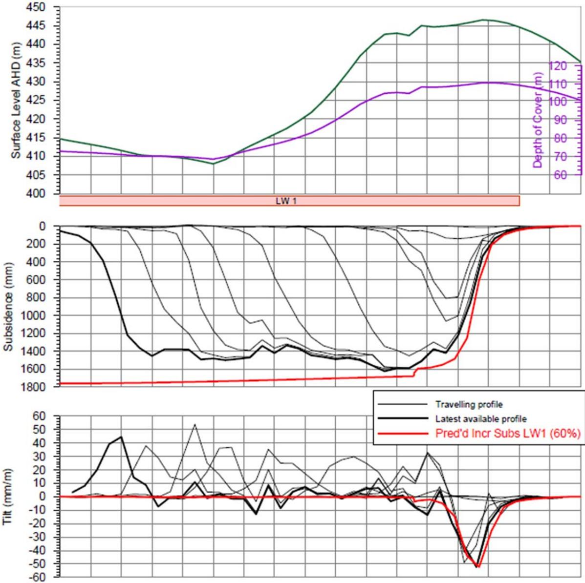
**Fig. 3.8 Ulan Coal Mine Monitoring Results along Longwall 1 (Permian Only)**
