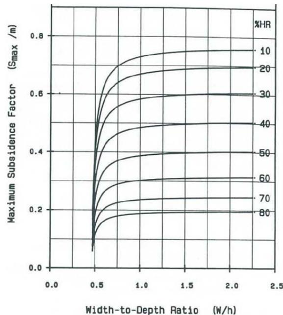
Fig. 3.3 Maximum subsidence factor versus Width to Depth Ratio curves (Karmis et al, 1987)
