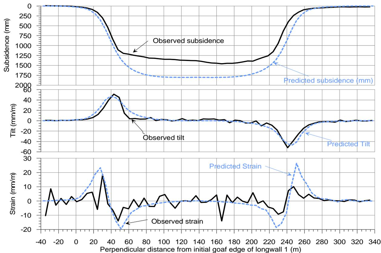
**Fig. 3.12 Beltana Mine Monitoring Results after extraction of Longwall 1 in Whybrow Seam – East Fence Cross Line**
