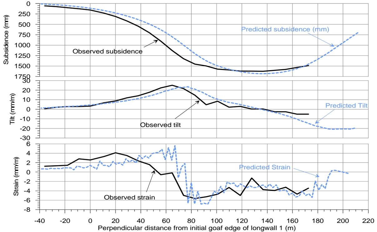
**Fig. 3.9 Beltana Mine Monitoring Results after extraction of Longwall 1 in Whybrow Seam – Ridge Cross Line**
