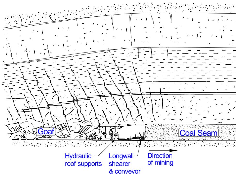
**Fig. 3.1 Cross-section along the Length of a Typical Longwall at the Coal Face**
