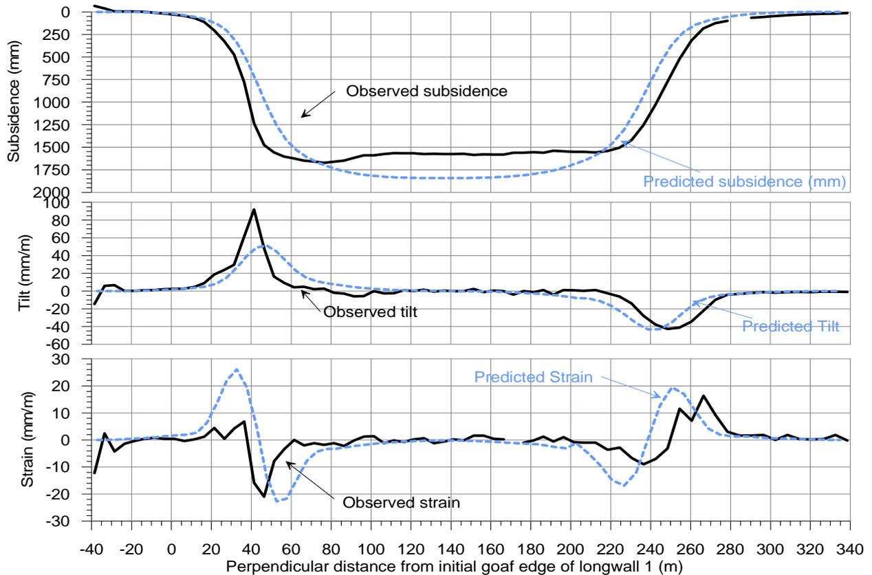
**Fig. 3.11 Beltana Mine Monitoring Results after extraction of Longwall 1 in Whybrow Seam – West Charlton Road Cross Line**
