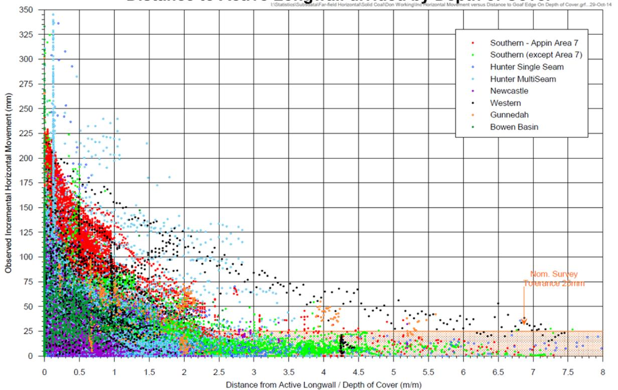
**Fig. 3.14** Observed Incremental Far-Field Horizontal Movements (mm) from many regions in NSW versus the distance to the nearest edge of the mined panel divided by the depth of cover (m/m)
