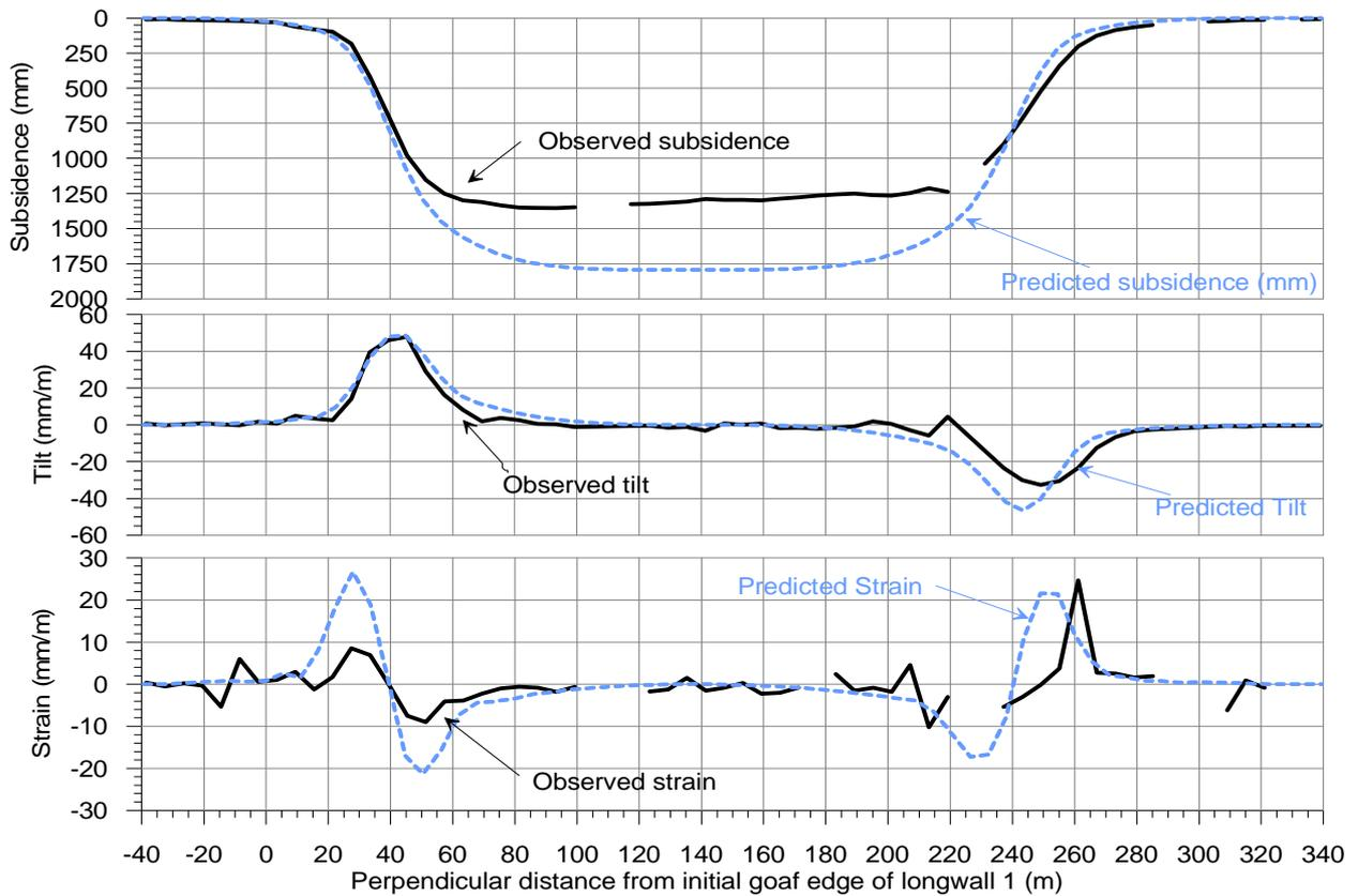
**Fig. 3.10 Beltana Mine Monitoring Results after extraction of Longwall 1 in Whybrow Seam – Optical Fibre Cross Line**
