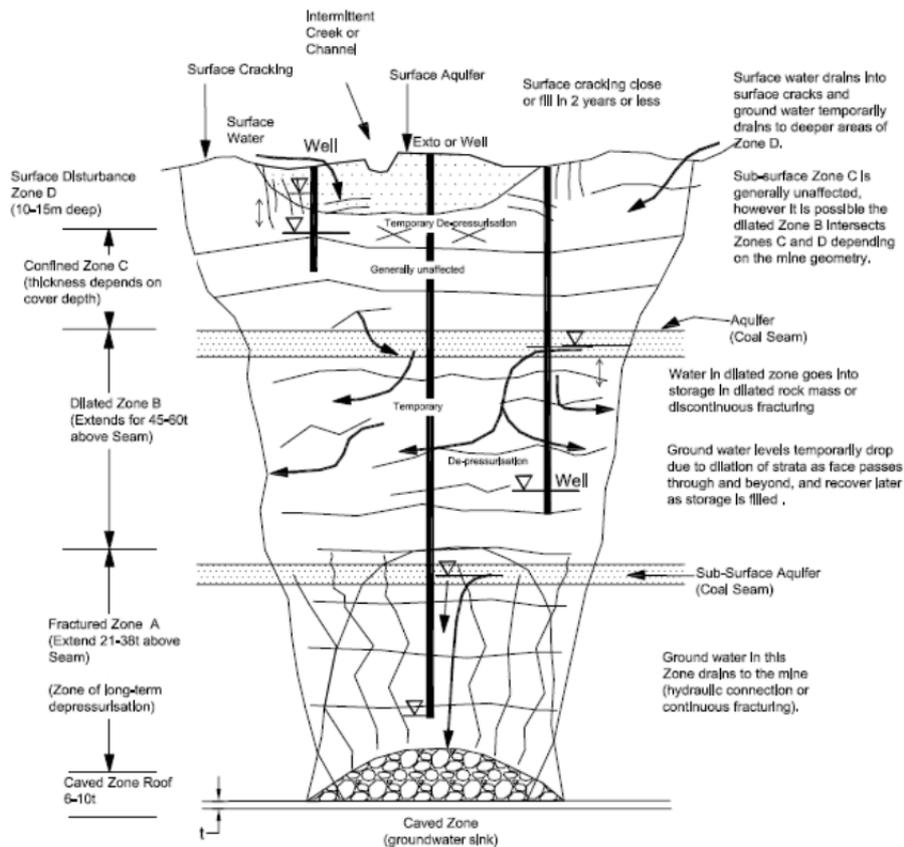
**Fig. 4.9 Zones in the Overburden according to Ditton (2005)**
