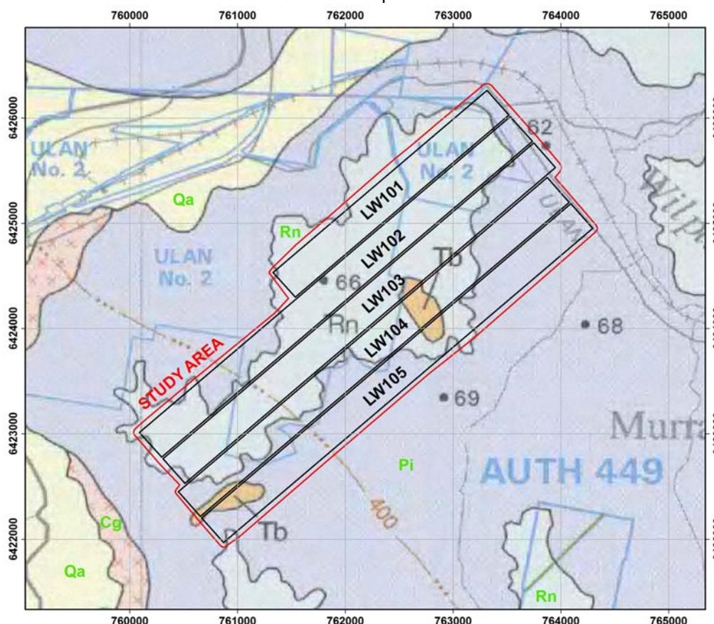
**Fig. 1.3 Surface Geological Map Showing the Proposed UG1 ModML Longwalls 101 to 105 and the UG1 Study Area** (Source-1:100000 Western Coalfield Map)
