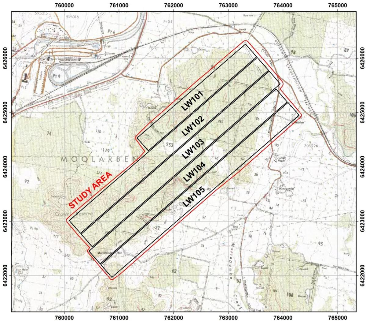
**Fig. 1.2 Topographic Map Showing Proposed UG1 ModML Longwalls 101 to 105 and the UG1 Study Area**
