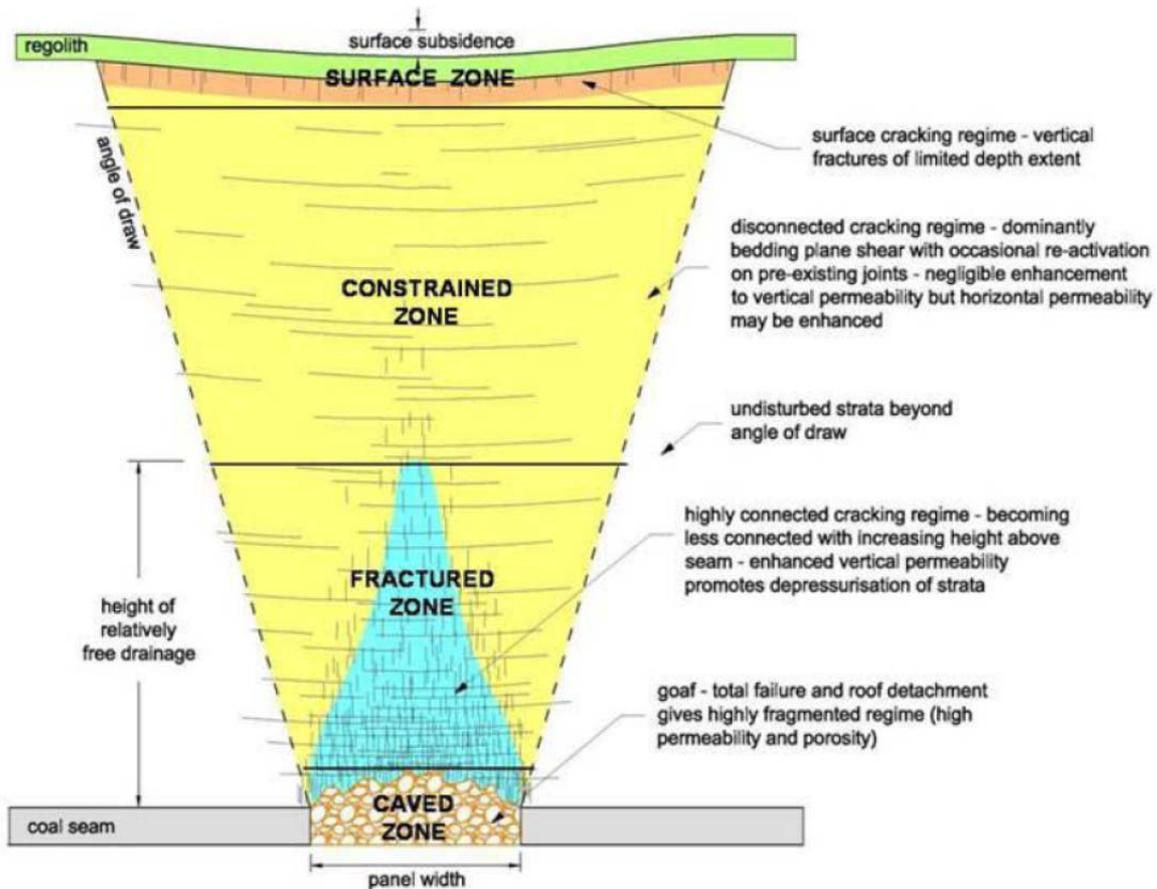
**Fig. 4.10 Zones and Nature of Overburden Fracturing - Conceptual Caving Model (Mackie, 2007)**
