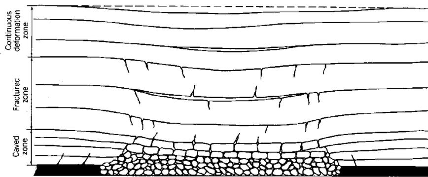
**Fig. 4.4 Zones in the Overburden According to Peng and Chiang (1984)**
