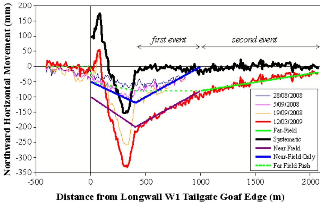
**Fig. 3.15 Components of horizontal movement inferred from measured subsidence profile (Mills)**
