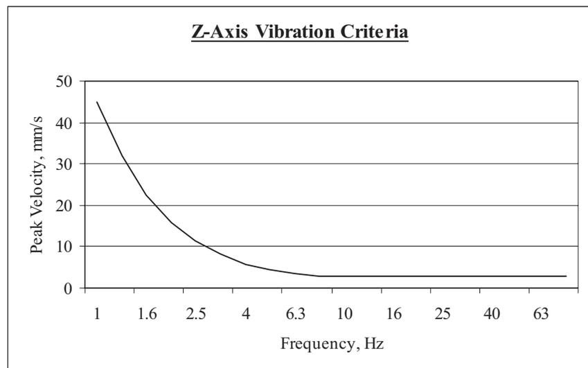
As train-induced ground vibrations typically comprise frequencies greater than 10Hz, and the vertical vibration criteria are more stringent than the horizontal vibration criteria, a maximum allowable vertical vibration velocity of 2.82mm/s applies.
