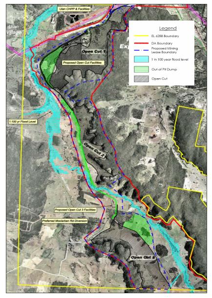
Figure 4: Open Cut Mine Components
