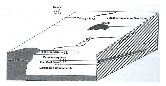
Figure 9: Conceptual Representation of the Hydrogeological Units in the Ulan Region<sup>2</sup>
