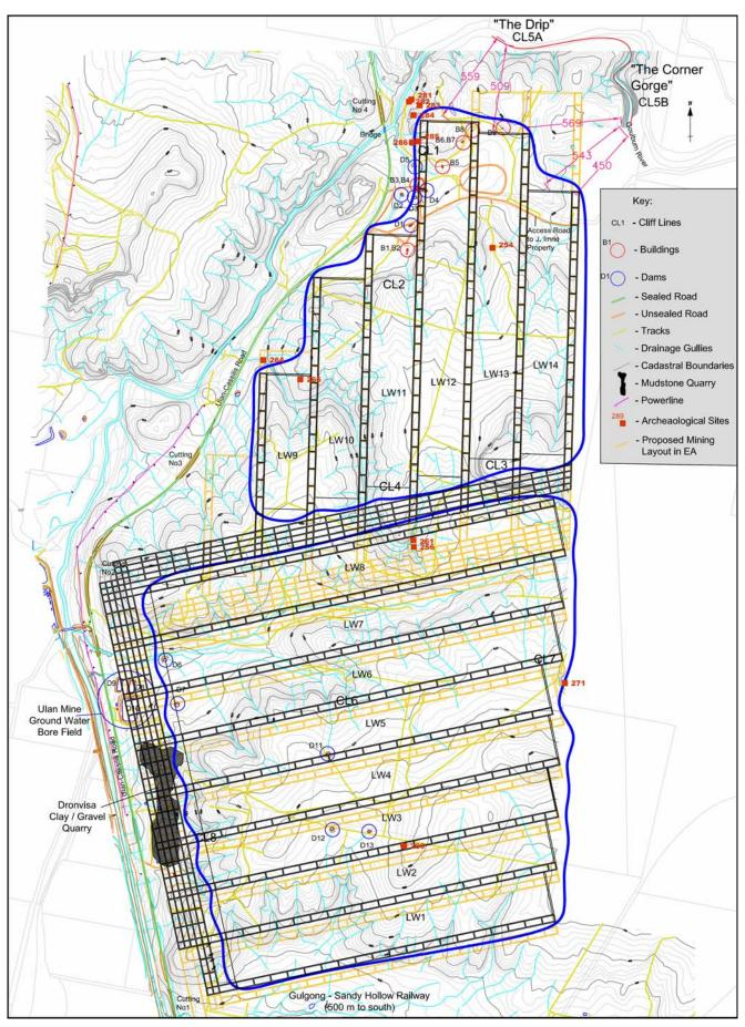
Figure 7: Proposed and Modified Underground Mine Layouts
